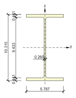
Figure 25: Beam cross-section
