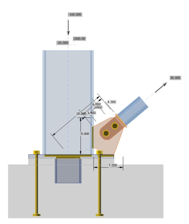
Figure 13: Gusset plate dimensions and loads on a transparent model
