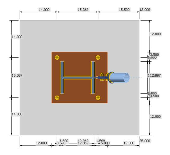
Figure 12: Concrete block dimensions
