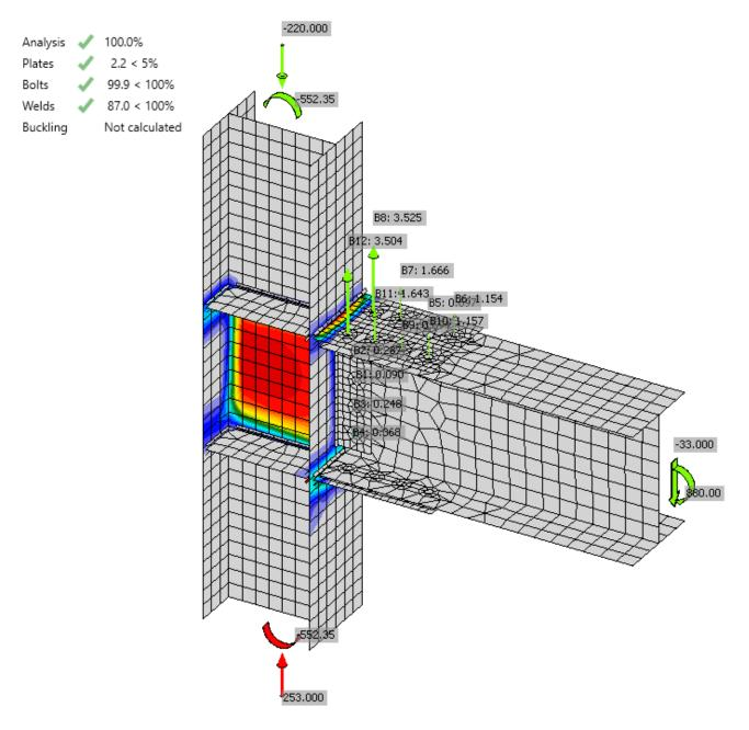
Figure 9: Plastic strain, loads and bolt forces at full utilization
