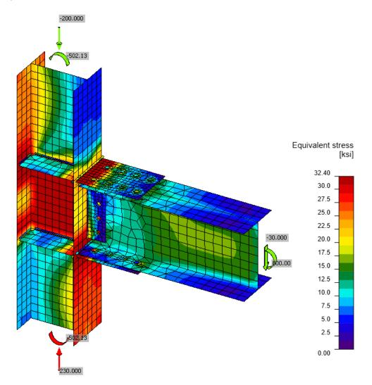
Figure 4: Von Mises stress
