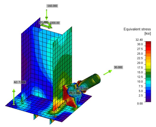
Figure 15: Von Mises stress
