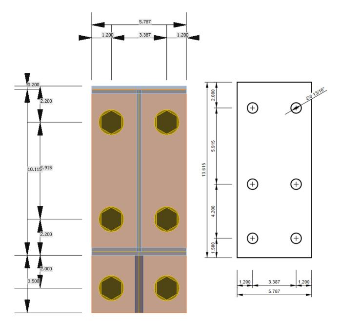
Figure 26: Dimensions of end-plate connection
