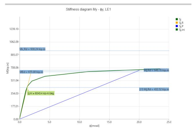
Figure 35: Stiffness of the joint
