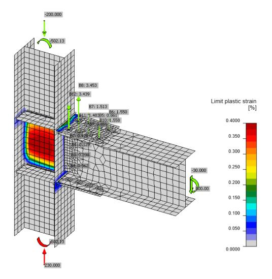
Figure 5: Plastic strain including the tensile forces in bolts
