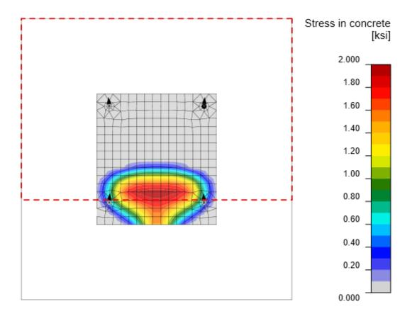
Figure 22: Stress in concrete under the base plate and area of concrete cone breakout
