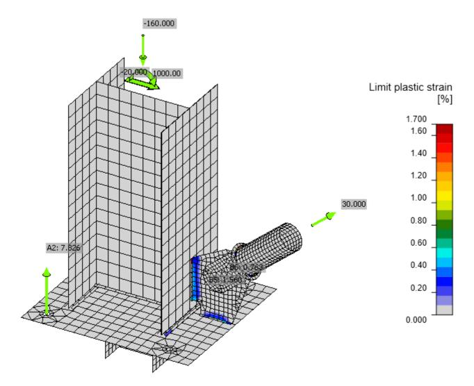
Figure 16: Plastic strain including the tensile forces in anchors
