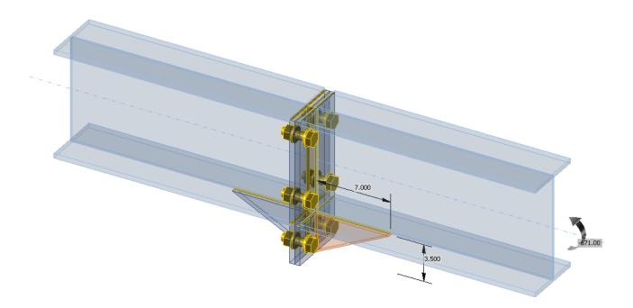
Figure 27: Transparent model with dimensions of widener and applied load
