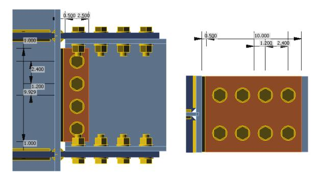
Figure 3: Geometry of fin plates
