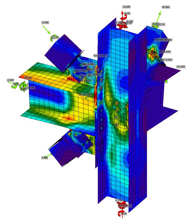
Figure 36: Complex joint analyzed in IDEA StatiCa Connection
