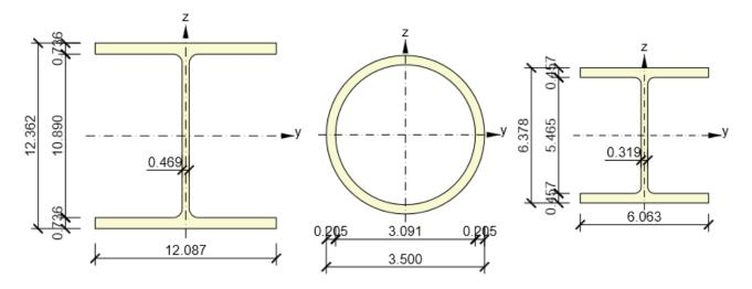
Figure 11: Cross-sections of column (left), brace (middle), and shear lug (right)
