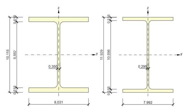
Figure 2: Cross-sections of column (left) and beam (right)
