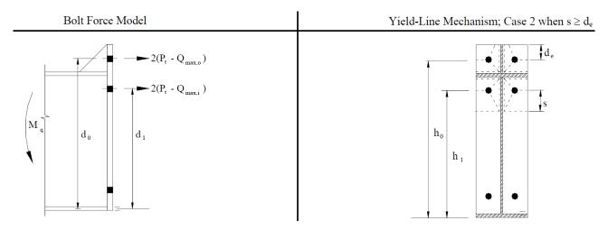
Figure 28: End-plate yield mechanism (Design guide 16)
