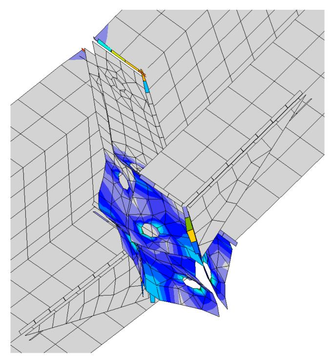
Figure 31: Detail of end plate deformation (scale  $20\times)$
