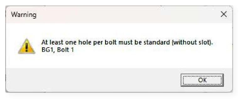
From the general part of the Theoretical Background: Bolts in standard holes can transfer shear force in all directions, bolts in slotted holes have one direction excluded and can move in this selected direction freely.
