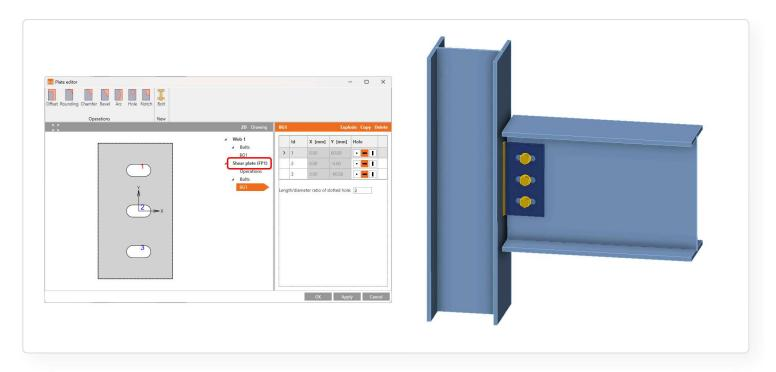
Variant 2: Slotted holes for a beam web
