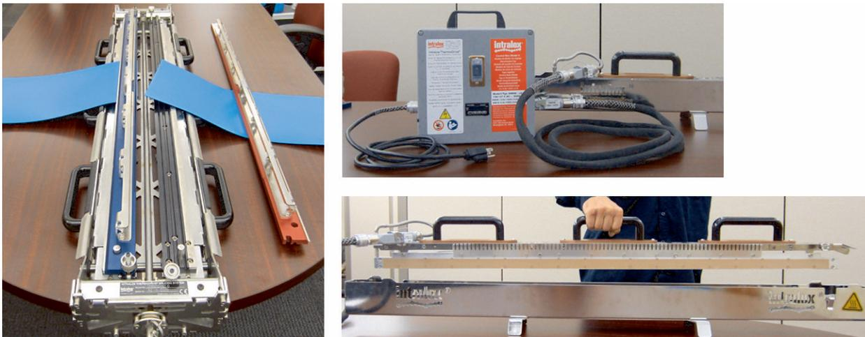
**Figure 19:** ThermoDrive Splicing System V2 and components
