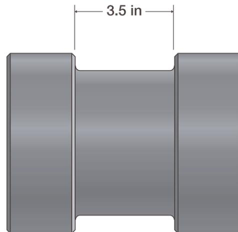
Figure 74: Roller inner dimensions
