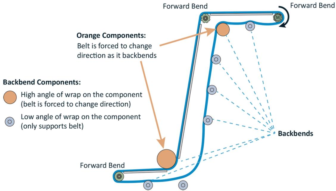
Figure 7: Sidewall backbends
