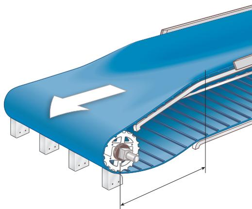
Figure 80: Correct transition distance
