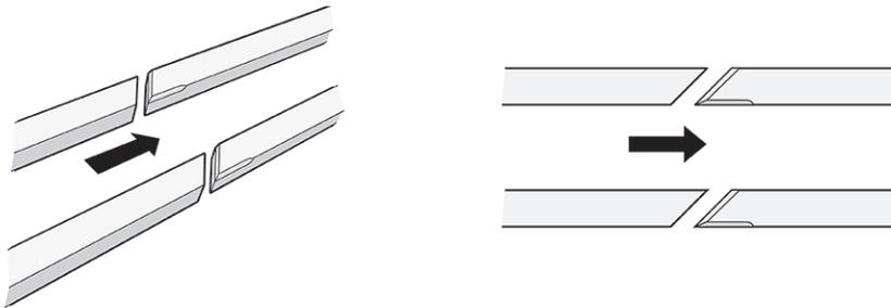
**Figure 31:** Rails chamfered at a 45-degree angle
