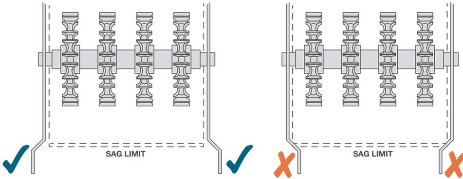
**Figure 39:** Correct steel brakes clearance
