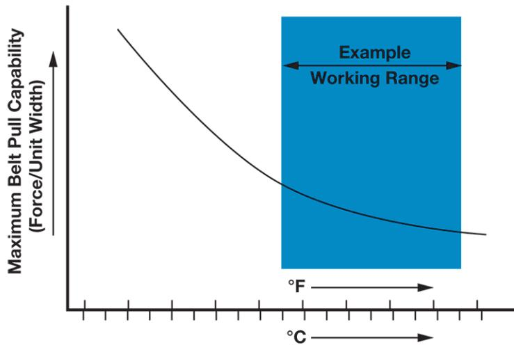
Figure 84: Temperature effects on maximum belt pull capability
