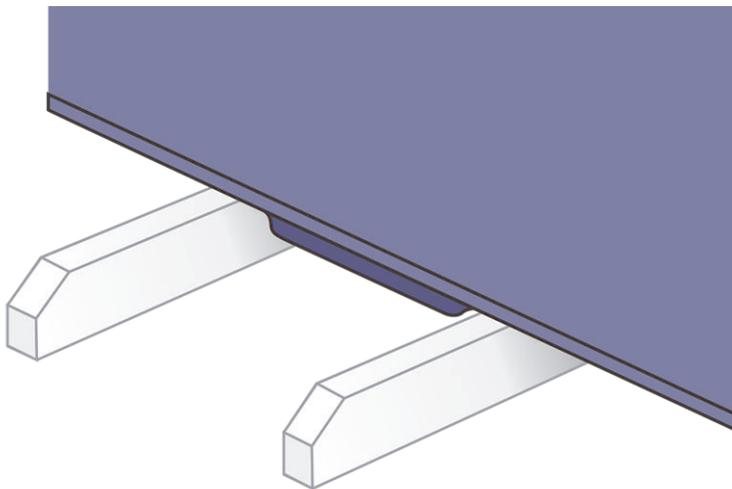
**Figure 77:** Lug alignment in gap between containment rails
