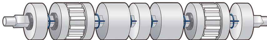
Figure 5: Spaced sprocket/support wheel (6 in wide square-bore sprocket)
