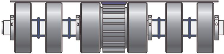
**Figure 3:** Spaced sprocket/support wheel (6 in wide sprocket)
