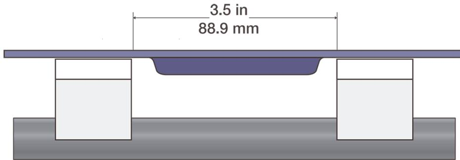
**Figure 75:** Single lug between containment rails
