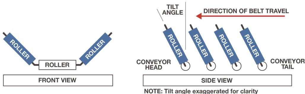
**Figure 66:** Tilt angles and direction of belt travel
