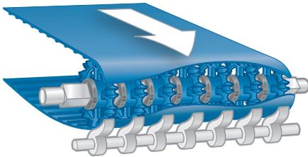
Figure 46: Outer sprockets installation
