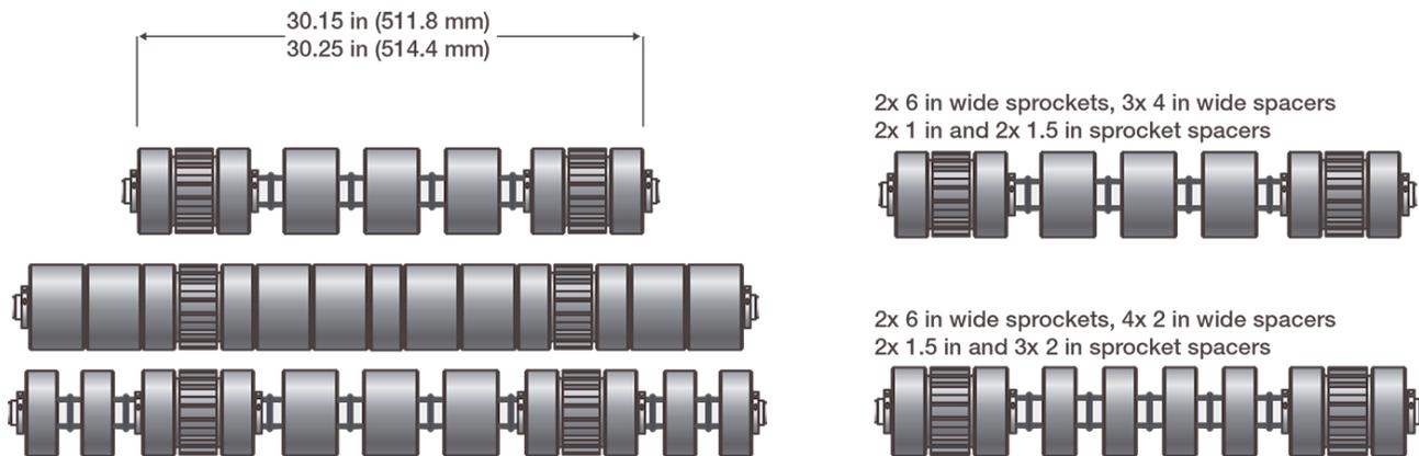
Figure 4: Drive sprocket and idle roller spacing
