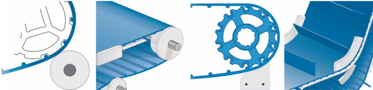
**Figure 24:** Components at or above the minimum bend radius
