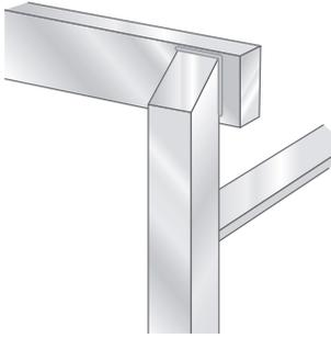
**Figure 28:** Correct joint assembly
