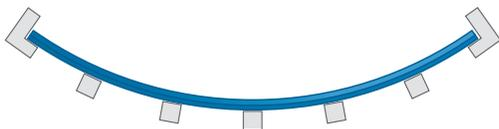
Figure 81: Belt with no trough groove
