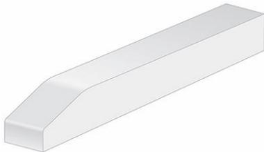
**Figure 32:** Wearstrip end chamfer
