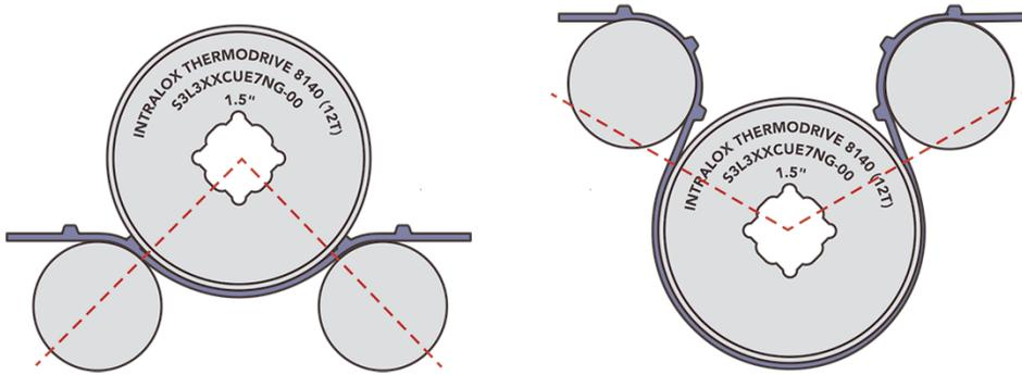
**Figure 71:** 90-degree and 225-degree belt-to-sprocket engagement
