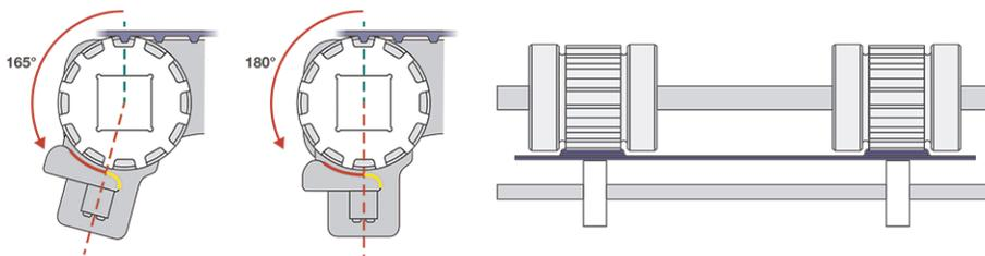
**Figure 72:** Position limiter placement between 165 degrees to 180 degrees
