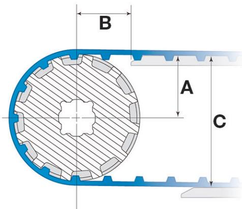
**A** Distance between the sprocket shaft centerline and the top of the carryway
