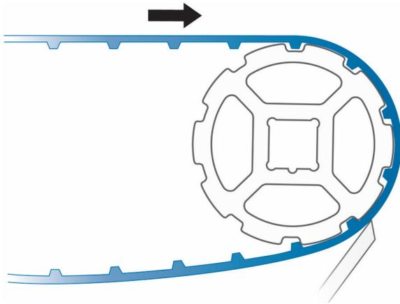
**Figure 56:** Scraper mounted at an angle
