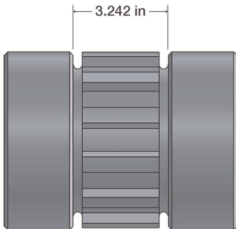
Figure 73: Sprocket inner dimensions
