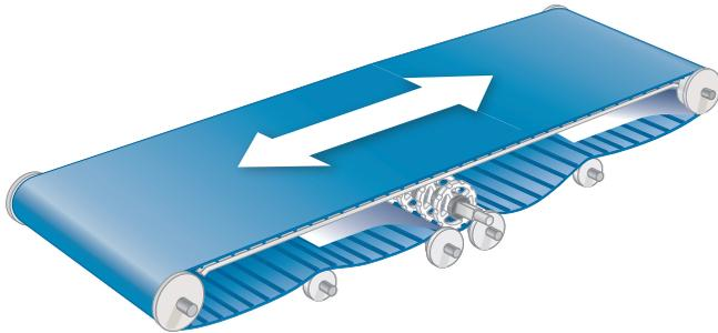
**Figure 54:** Center drive sprocket and position limiter locations
