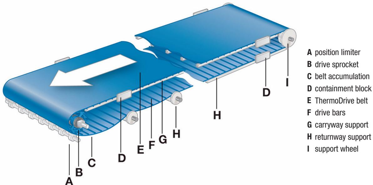
**Figure 26:** Conveyor belt components
