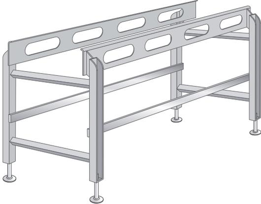
**Figure 27:** Simple structure to provide open access for sanitation
