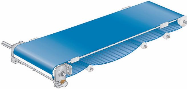
**Figure 37:** Catenary sag between components
