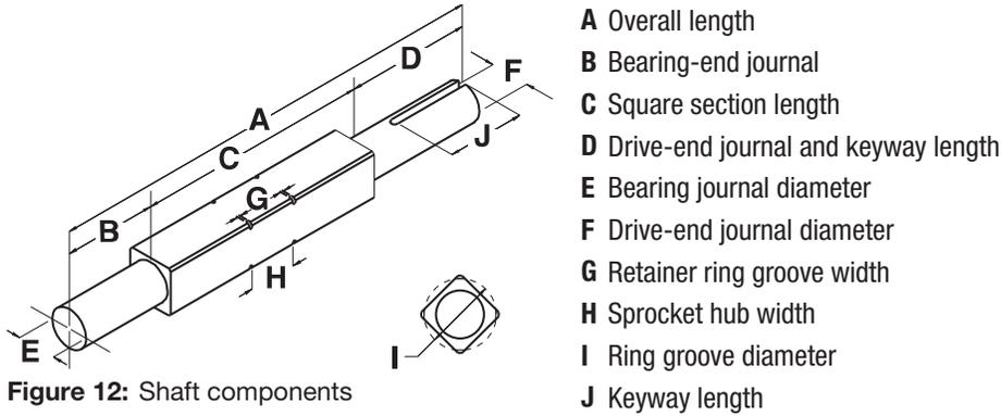
Figure 12: Shaft components
