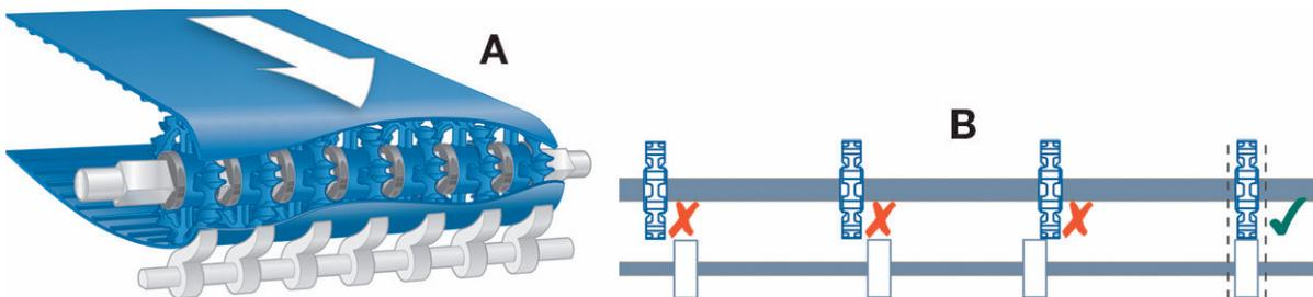
**Figure 52:** Correct alignment and minimum clearance for belts without accessories
