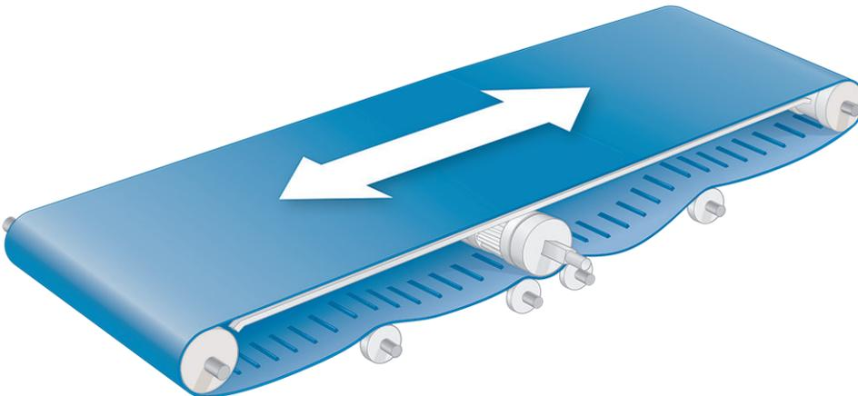
**Figure 70:** Center drive sprocket and position limiter locations
