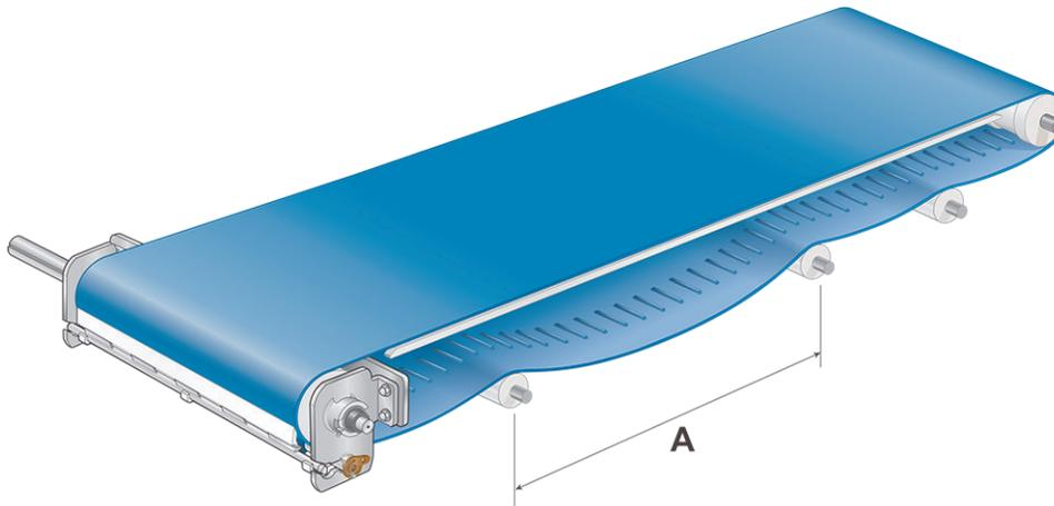
**Figure 68:** Correct support spacing
