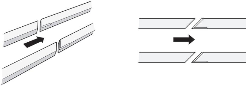
**Figure 65:** Rails chamfered at a 45-degree angle
