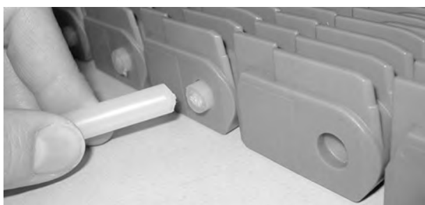
Figur 217: Skyv pinnen forbi Shuttleplug
