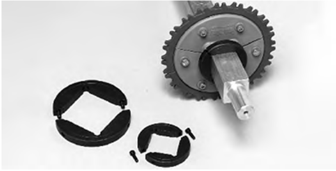
Figure 90: Split collar retainer rings
