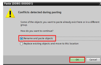
Figure 24: Paste Warning When Adding More Than One ISC CAM PLC tags to a Project
