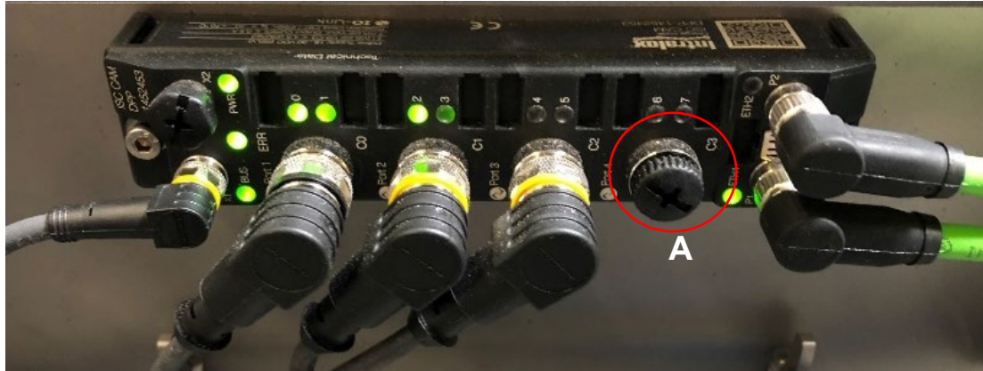
Figure 1: Hardwire signal connections
