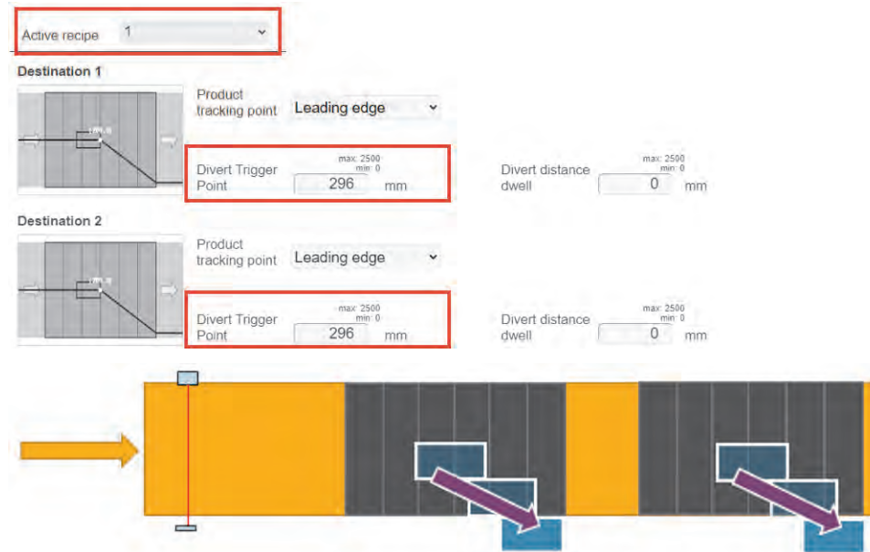
Figure 90: Recipe 1 – Smaller product, larger divert trigger point
