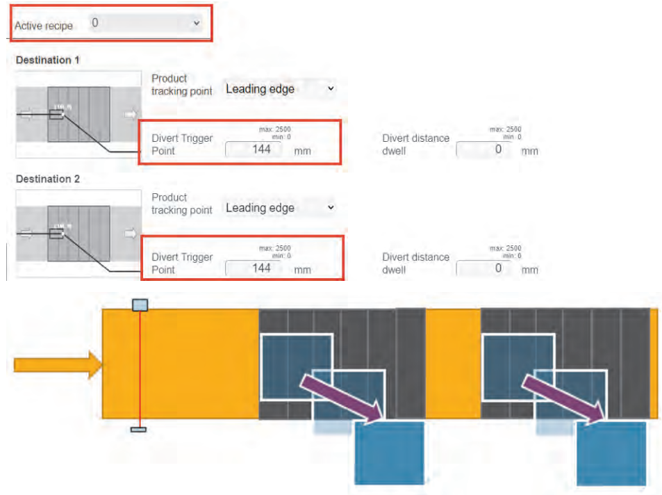
Figure 89: Recipe 0 – Larger product, smaller divert trigger point
