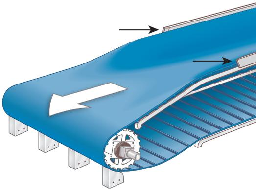
Figure 40: UHME-PE containment rails
