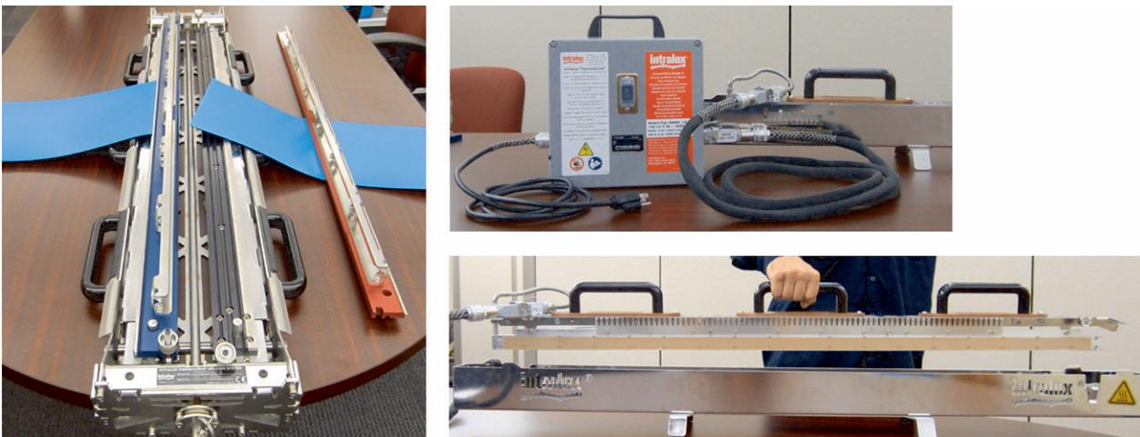
**Figure 56:** ThermoDrive Splicing System V2 and components
