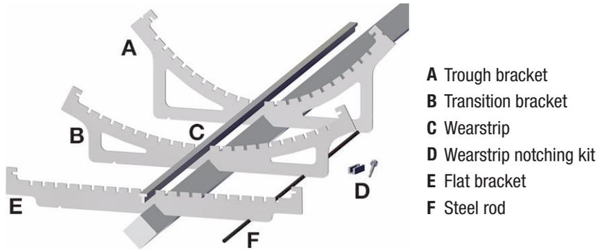
**Figure 55:** Trough converter components
