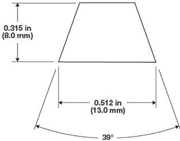
Figure 45: V-guide nominal geometry
