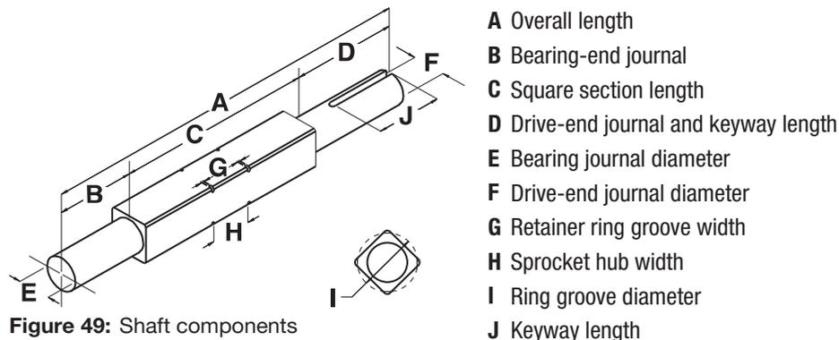
Figure 49: Shaft components
