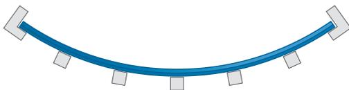
Figure 42: Belt with no trough groove
