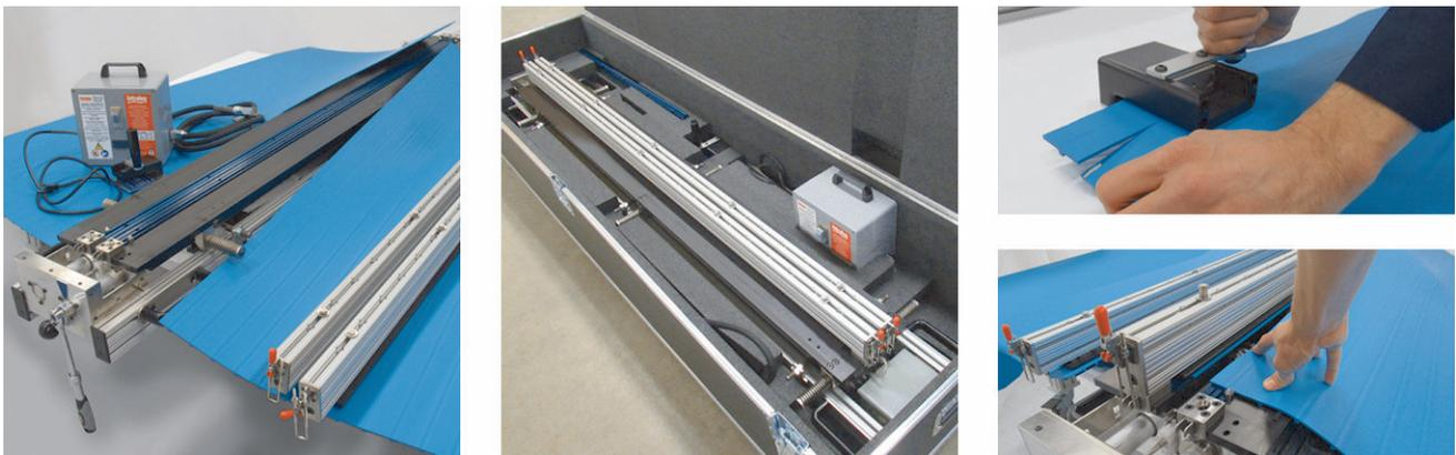
**Figure 57:** ThermoDrive Streamline Splicing Set and components
