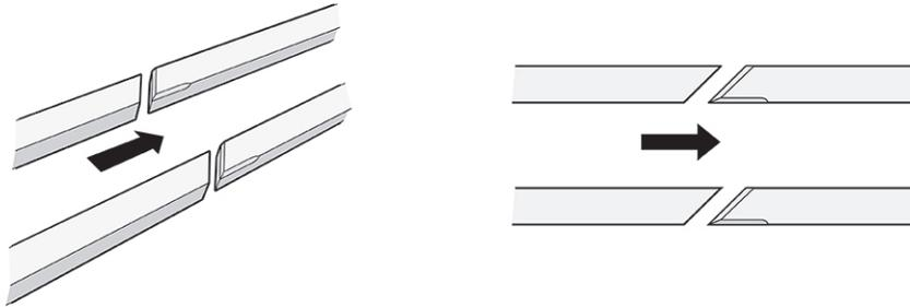
**Figure 24:** Rails chamfered at a 45-degree angle
