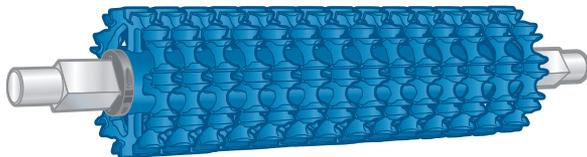
**Figure 12:** Stacked sprockets
