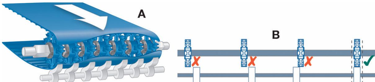
**Figure 15:** Correct alignment and minimum clearance for belts without accessories
