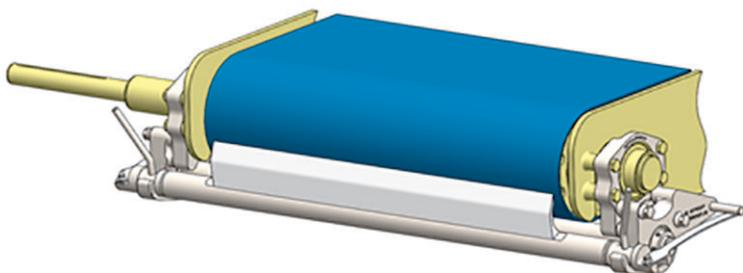
**Figure 53:** TD Drive Components (end drive)
