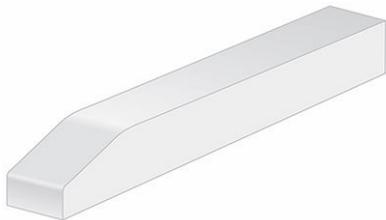
**Figure 25:** Wearstrip end chamfer
