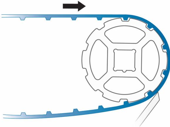
**Figure 20:** Scraper mounted at an angle
