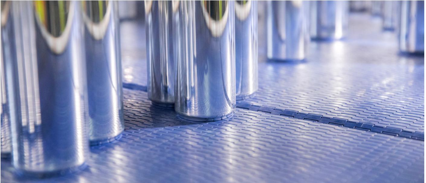
Intralox® Series 560 belting offers an exceptional tight transfer solution for mass can conveyance. Eliminating the need for dead plate transfers, S560 belting has been shown in field testing to reduce spoilage of 12-oz sleek cans by 70% compared to transfers with dead plates. S560 belting also prevents cans from becoming stranded on dead plates, reducing the risk of palletizing mixed labels and eliminating labor needed to clear the line of stranded cans at each label change.
