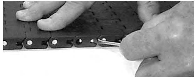
Figure 166: Fermez le Slidelox
