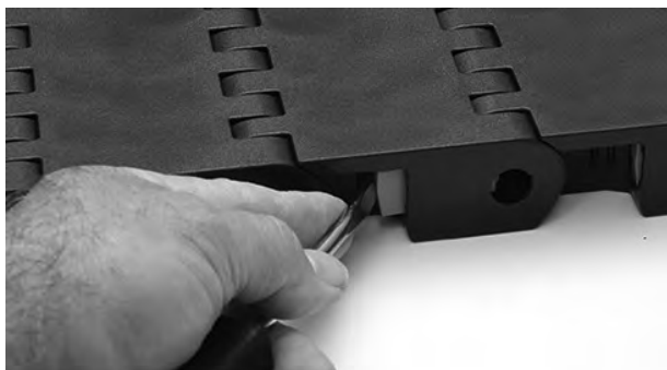
Figure 261: Fermez le Slidelox
