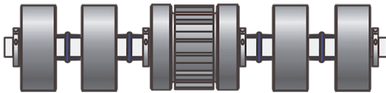
Figure 1: Spaced sprocket/support wheel (6 in wide square-bore sprocket)
