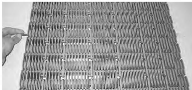
**Figura 218:** Abra o Shuttleplug
