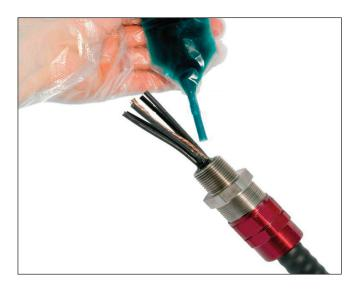
seal. The RapidEx resin adheres to both the cable conductors and the inside of the barrier tube, creating a bond that is set for the life of the cable gland product.
